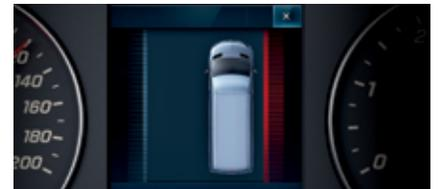
**ACTIVE LANE KEEPING ASSIST<sup>8</sup>** provides visual and audible warnings if your vehicle leaves its lane unintentionally. A camera in the windshield monitors the road ahead and helps detect when you may have unintentionally veered from lane markings.
