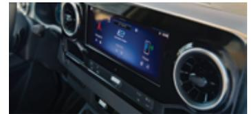
**10.25" MBUX TOUCHSCREEN,** activated via touch, voice control, or touch buttons on the steering wheel, is available in the Sprinter.
