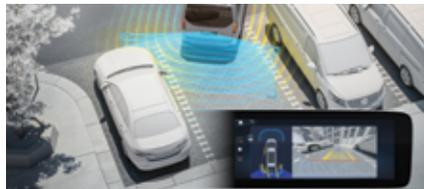
**PARKING PACKAGE<sup>7</sup>** uses twelve distance sensors and the reversing camera to support you while parking in confined spaces or driving out of exits. It warns you of objects around the vehicle, limits speed when driving off if obstacles are detected ahead, and displays dynamic guidelines when using the reverse gear.
