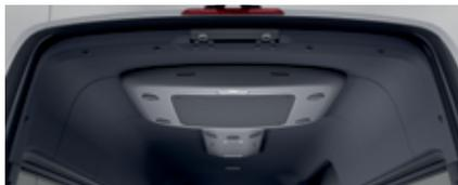
Roof air conditioning comes in two output levels, including a high-performance air conditioner.
