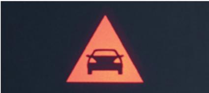
**ACTIVE BRAKE ASSIST<sup>2</sup>** senses the likelihood of a collision with a vehicle ahead, and sends both a visual and audible warning; autonomous braking can also be initiated.
