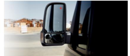
**BLIND SPOT ASSIST<sup>4</sup>** uses radar sensors to monitor the area behind and next to your vehicle - if a vehicle is detected, a visual warning will appear in the exterior side mirror. The system's Rear Cross-Traffic Alert (RCTA)<sup>5</sup> employs automatic braking to avoid a collision with traffic that is crossing the vehicle's path (e.g., vehicles or pedestrians) when reversing.
