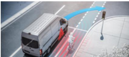
**SIDEGUARD ASSIST<sup>6</sup>** provides visual and acoustic warnings while turning when a road user (e.g., cyclist) enters a defined area on the passenger side.
