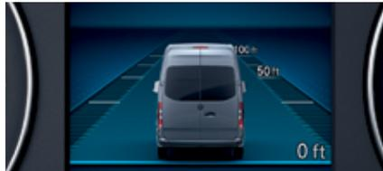
**ACTIVE DISTANCE ASSIST DISTRONIC<sup>3</sup>** is an intelligent cruise control system that senses traffic conditions and actively controls your speed to keep you at a set distance.
