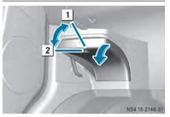
Fuse box in the footwell on the left-hand side of the vehicle.
