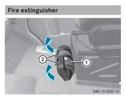
Fire extinguisher at the front of the base of the codriver's seat
