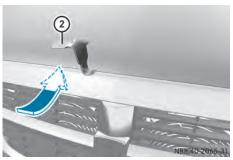
Push hood catch release handle (2) upwards.
