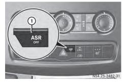
Press button ①. When ASR is deactivated, the warning lamp in the instrument cluster lights up.
