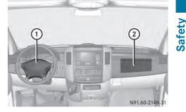
Driver's front air bag ① deploys in front of the steering wheel; co-driver's front air bag ② deploys in front of and above the glove box. They are deployed:
