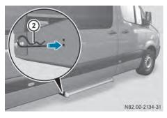
Insert R-clips (2) into the step as far as they will go through the holes on both sides of the housing.
