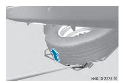
Use the pump lever to lift the spare wheel beyond the rear edge of the spare wheel carrier.
