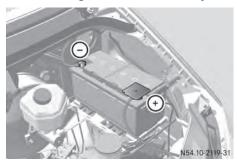
Additional battery in the engine compartment
