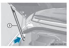
Swing the hood upwards until support strut
