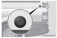
With the rear door opened to an angle of 270°, push it against magnetic door retainer (2) on the side wall.
