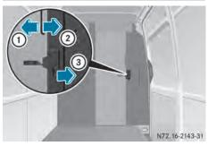
► **To unlock:** press the catch in the direction of arrow ③.
