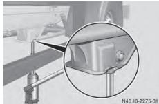
Jacking point (example: Cab Chassis)
