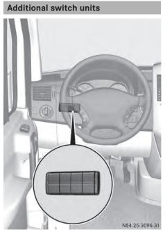
Switch unit between the light switch and the steering wheel
