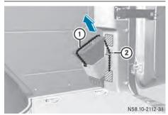
Wheel chock in the load/passenger compartment
