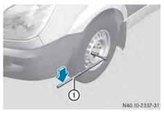
Loosen the wheel nuts or wheel bolts on the wheel to be changed by about one turn using extended lug wrench ①. Do not unscrew the wheel bolts or wheel nuts completely.
