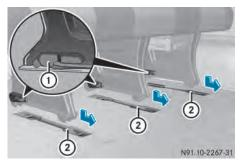
Examine seat mounting recesses (2) on the vehicle floor.
