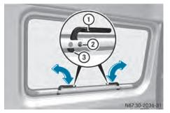
► **To open:** turn both handles ① to a vertical position. Locking pins ② will break in the process.
