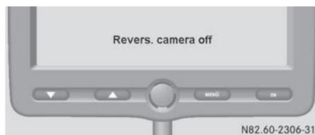
If you drive faster than 6 mph (10 km/h), the monitor switches off automatically for safety reasons.
