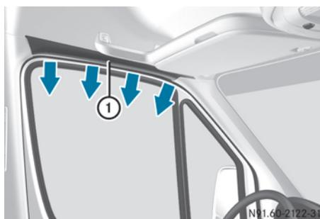
Window curtain air bags (1) enhance protection for the head (but not the chest or arms) of the vehicle occupants on the side of the vehicle on which the impact occurs.
