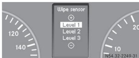
You can use the **Wipe sensor** function to set the sensitivity of the rain/light sensor.
