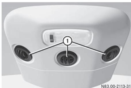
On vehicles with rear-compartment air conditioning, adjustable air vents are integrated into the roof duct.
