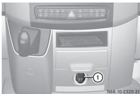
Socket on the lower section of the center console
