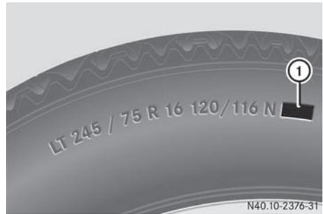
In addition to the load-bearing index, load rating **(1)** may be imprinted after the letters that identify speed rating on the sidewall of the tire (▷ page 290).
