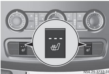
The three red indicator lamps in the
