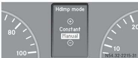
For safety reasons, it is only possible to change this setting when the vehicle is stationary. The factory setting is **Constant** in countries in which daytime running lamp mode is mandatory.
