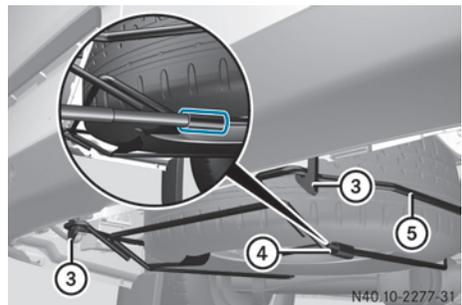
Spare wheel carrier under the vehicle
