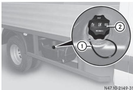
The DEF reservoir on the right-hand side of the vehicle (example: Chassis Cab)
