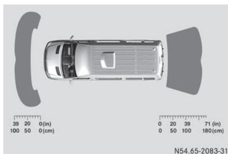
The sensors must be free of dirt, ice or slush. Otherwise, they cannot function correctly. Clean the sensors regularly, taking care not to scratch or damage them (▷ page 259).
