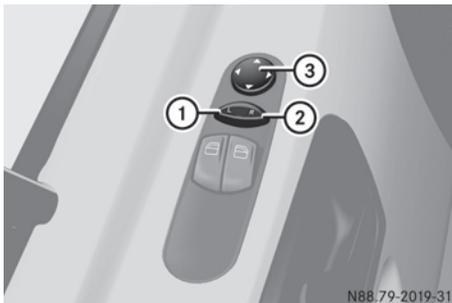
Button and switch for mirror adjustment
