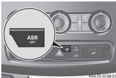
When ESP® is intervening and the
