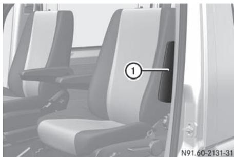
Thoraxbags (1) are only installed for individual seats in the outer seat cushions of the driver's and co-driver's seats.
