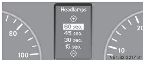
In the **Headlamps** submenu, you can set whether and for how long you wish the exterior lighting to remain on after closing the doors.
