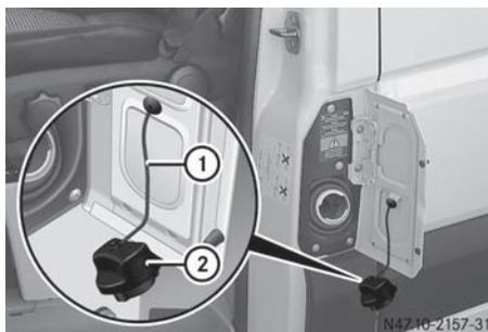
The fuel filler flap is beside the front left-hand door when viewed in the direction of travel. It is only possible to open the fuel filler flap when the front door is open.
