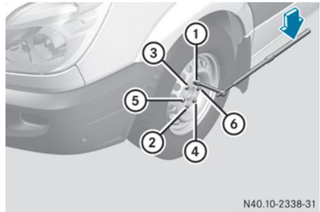
Tightening torque pattern
