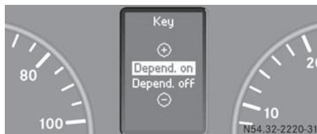
The **Key** function allows you to define whether settings for some submenus are stored with a key dependence.
