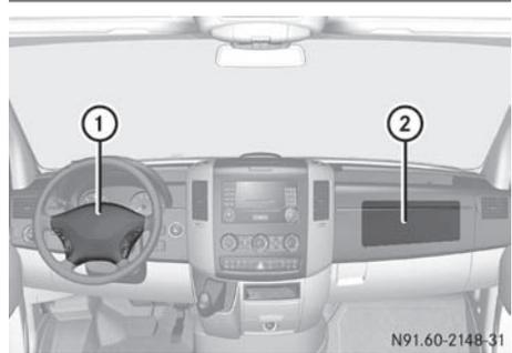
Driver's air bag ① inflates in front of the steering wheel; co-driver's front air bag ② inflates in front of and above the glove box and center console.
