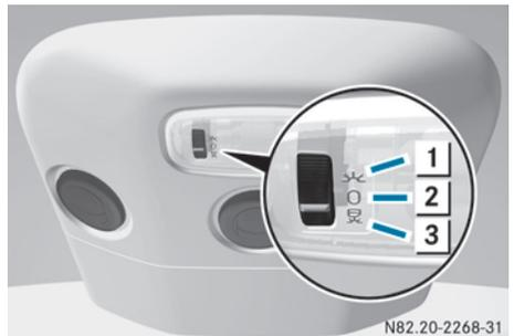
Interior light with switch (example: Passenger Van with rear-compartment air conditioning)
