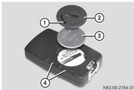
► Remove battery cover **②** using a suitable implement, e.g. a coin, by turning it counter-clockwise.
