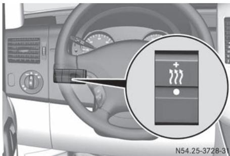
At an outside temperature of up to 39 °F(4 °C) the fuel-fired heater booster system heats the vehicle interior as quickly as possible when the engine is running.
