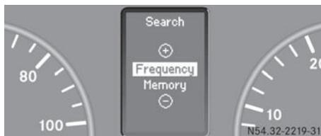
With the **Search** function, you can set how the radio changes the station when you operate it with the steering wheel buttons (not with Audio 20).
