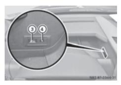
PND connector (on the side behind the instrument cluster)
