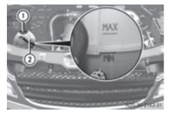
Example: cap and coolant expansion tank
