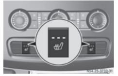
The three red indicator lamps in the ## button show the activated heating level 1 to 3.
