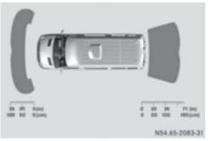
The sensors must be free of dirt, ice or slush. Otherwise, they cannot function correctly. Clean the sensors regularly, taking care not to scratch or damage them ( $\triangleright$  page 268).
