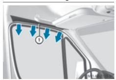
Window curtain air bags (1) are integrated into the side of the roof frame above the front doors.
