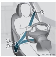
▶ Press release button ①, hold belt tongue ② firmly and guide it back towards belt outlet ③.
