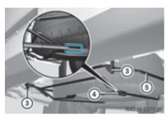
Spare wheel carrier under the vehicle
