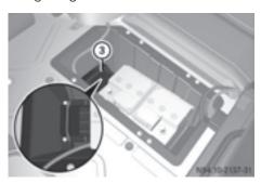
► Loosen the bolts holding retainer (3), which prevents the battery from moving around.
