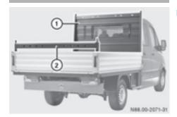
Example: ladder rack on Chassis Cab
