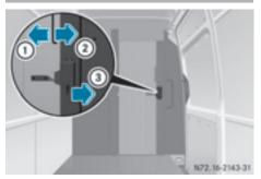
▶ To unlock: press the catch in the direction of arrow (3).
