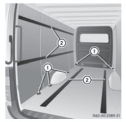
Cargo tie-down point (example: Cargo Van with loading rails)
