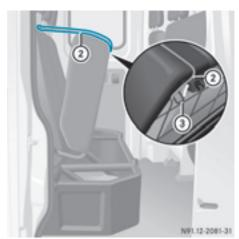
Retainer loops (2) are secured to the outer head restraints.
