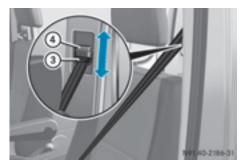
The shoulder section of the belt must always run over the center of the shoulder. Adjust the belt outlet if necessary.
