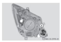
► Bi-Xenon headlamps: turn bulb holder with bulb ② counter-clockwise and remove it.
