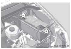
Additional battery in the engine compartment
