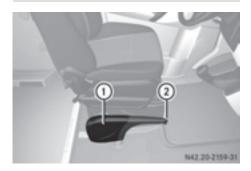
The brake lamps are not illuminated when you brake the vehicle using the parking brake. As a rule, you may only apply the parking brake when the vehicle is stationary.
