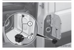
The fuel filler flap is on the left side of the vehicle behind the front door. It is only possible to open the fuel filler flap when the front door is open.
