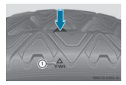
Marker (1) shows the location where the bar indicator (arrow) for tread wear is integrated into the tire tread.
