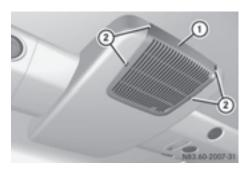
Filter magazine, located on the roof in the rear compartment
