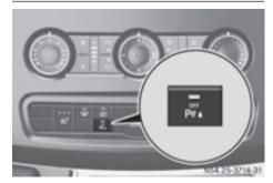
▶ Press the button. If PARKTRONIC is deactivated, the indicator lamp in the switch lights up.
