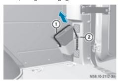
Wheel chock in the load/passenger compartment
