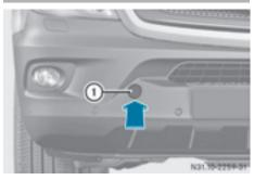
The fixture for the front towing eye is located in the bumper.
