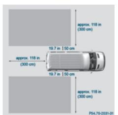
Blind Spot Assist monitors the area approximately 10 ft (3.0 m) behind your vehicle and approximately 1.6 ft (0.5 m) to 11.5 ft (3.5 m) each side of it. For this purpose, Blind Spot Assist uses radar sensors in the rear bumper
