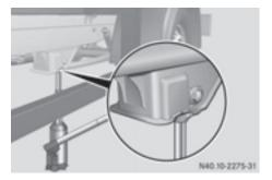
Jacking point, rear axle (example: Cab Chassis)
