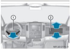
Driver's air bag (1) deploys in front of the steering wheel. Front-passenger front air bag (2) deploys in front of and above the glove box and the center console.
