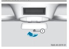
► Anti-glare mode: push anti-glare lever (1) in the direction of the arrow.
