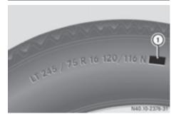
In addition to the load-bearing index, load rating 1 may be imprinted after the letters that identify speed rating on the sidewall of the tire ( $\triangleright$  page 300).
