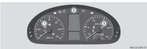
Instrument cluster in vehicles with steering-wheel buttons
