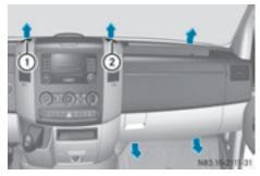
Air vents (example: right-hand side of the vehicle)
