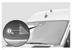
1 Lane Keeping Assist camera Lane Keeping Assist supports you from speeds of approximately 40 mph(60 km/h).
