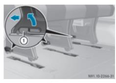
Locking mechanism lever on the feet of the bench seat
