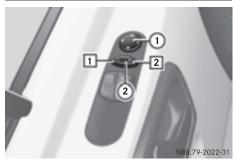
Adjustment buttons and switches for setting the mirrors
